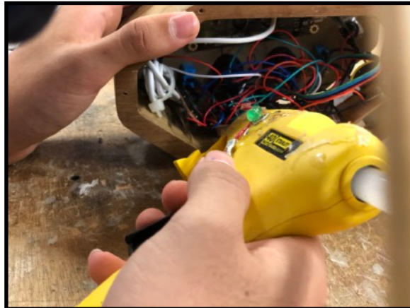
Fig. 3 Hot gluing the circuit to the balsa pieces
