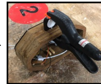
Fig. 9 - Clamping the charger to the main body and letting it dry
