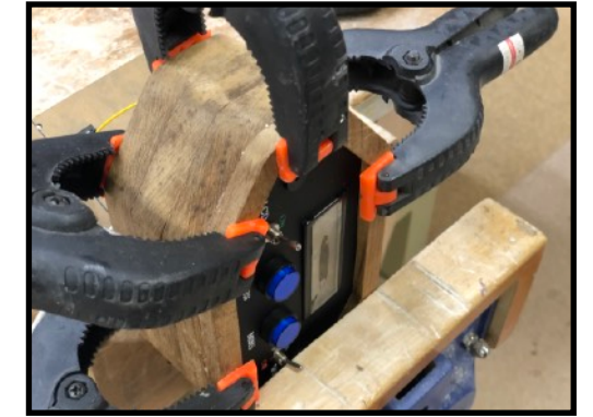
Fig. 9 Clamping the body to let the glue dry
