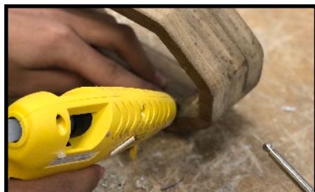
Fig. 9 - Hot gluing the balsa wood into the body
