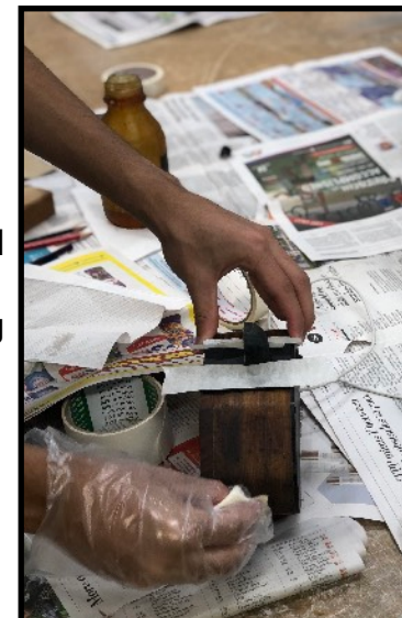
Fig. 8 Applying teak oil
