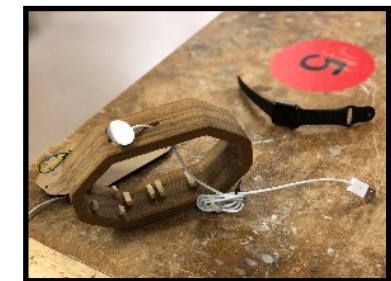
Fig. 7, 8. Making sure the charger fits and gluing it to it's housing
