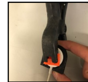
Fig. 7, 8. Making sure the charger fits and gluing it to it's housing
