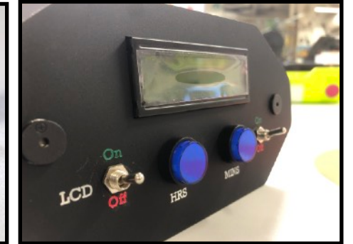
Fig. 4 - Front of interface after all components have been attached
