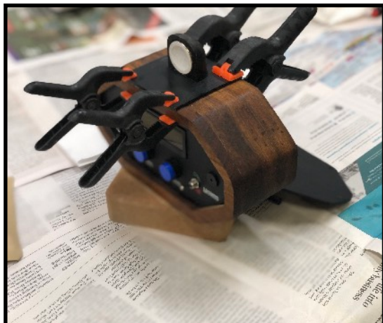
Fig. 2 Clamping the acrylic piece as it dries
