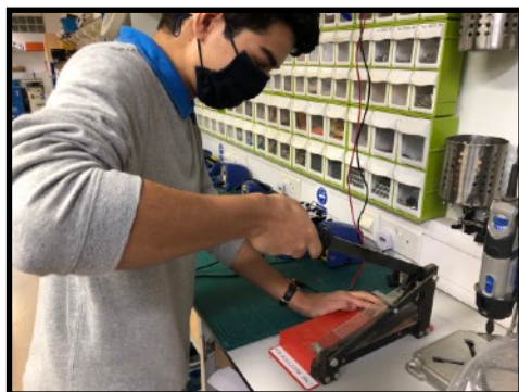
Fig. 5 - Using the PCB Guillotine to cut the perfboards (make sure fingers are not near the blade)
